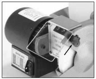
Figure 1. Knob to adjust eye shield.
